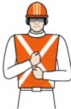
Travel both tracks (crawler cranes only)
