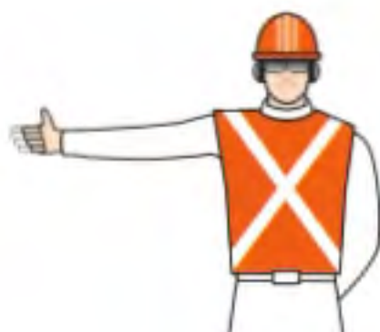
Raise boom and lower load (flex fingers)
