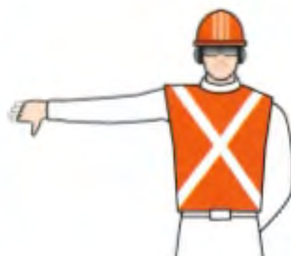
Lower boom and raise load (flex fingers)
