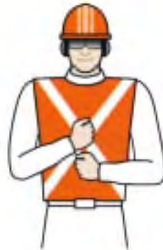
Travel both tracks (crawler cranes only)
